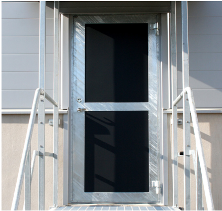
Hot-dip galvanised door leaf frame, clad with polyester coated sheet metal according to the customer's choice of colour.
