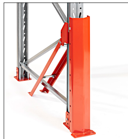
Upright reinforcement 90/110 high mod front - to be fitted in front of the upright. Provides the best possible protection for the most exposed part of the frame. Height 760 mm.
