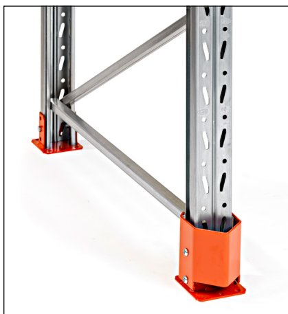
Upright reinforcement 90/110 low mod. - to be fitted together with the sleeve footplate. Provides excellent protection for the upright frame member, without taking up extra space. Height 150 mm.
