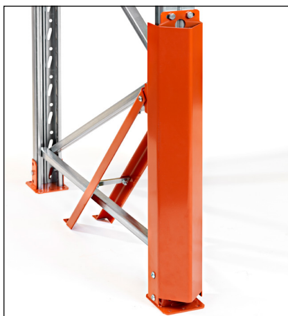
Upright reinforcement 90/110 high mod - to be fitted with the sleeve footplate. Provides the best possible protection for the most exposed part of the frame. Height 760 mm.
